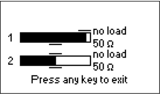
For the 50-Ohm load, the filled bars should stand at corresponding positions (notice the “no load” and “50 Ω” marks):
