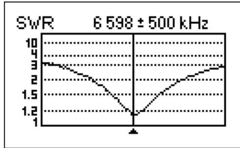
You may set the center frequency (the **2** key) or scanning range (the **3** key). By using arrow keys, these parameters may be increased or decreased.
