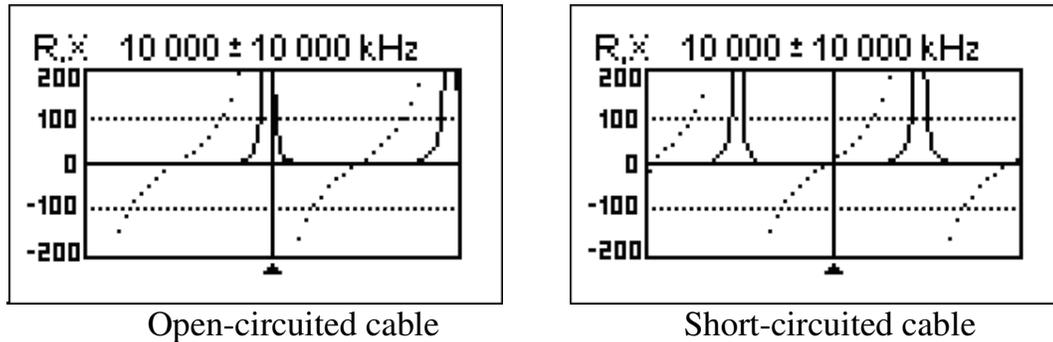
The above pictures show R and X graphs for a piece of cable with open- and short-circuited end. A *resonant frequency* is a point at which X (see the dotted line) equals to zero:
