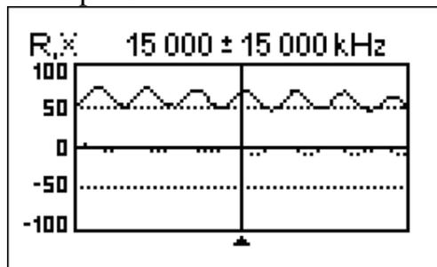
3. Changing the display range and performing additional scans, find a frequency where R (solid line) reaches its maximum, and another frequency with minimum. At these points, X (dotted line) will cross the zero line.
