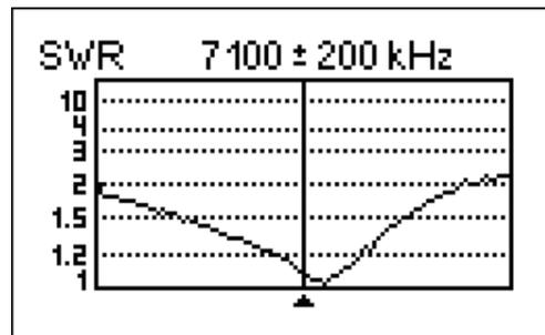
The above picture shows SWR graph of an HF antenna. The operating frequency is 7.1 MHz. The SWR at this frequency is about 1.1, which is acceptable.
