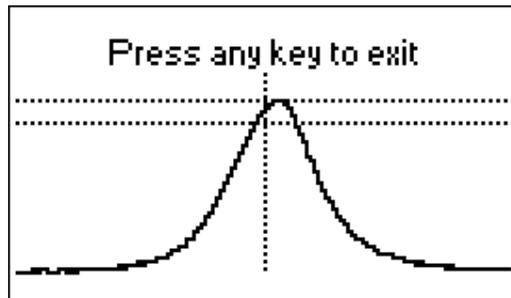
The top of the curve should be located in the middle of the screen, between the two horizontal dotted lines. A small horizontal shift of the curve is allowed.
