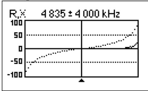
The 1/4-wave resonant frequency of the piece of open-circuited RG-58 cable is 4835 kHz
