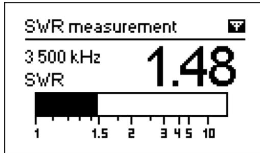
Set the desired frequency (the **2** key) or change it with left or right arrow keys.
