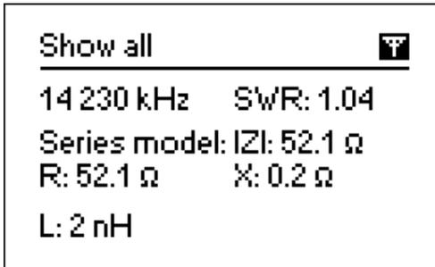
For this mode, you may choose either *series* or *parallel* model of impedance of a load through the *Settings* menu:
