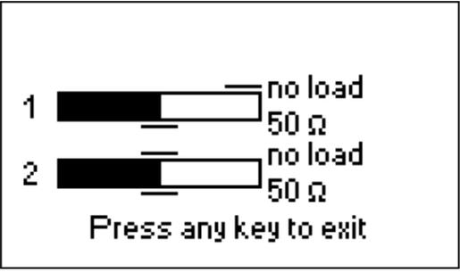
If the bars are not filled at all, the RF output stage or/and the detector are not working properly in the analyzer.
