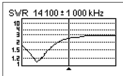
The actual resonant frequency is about 13.4 MHz, which is too far from the desired one. The SWR at 14.1 MHz is about 2.5, which is not acceptable in most cases.
