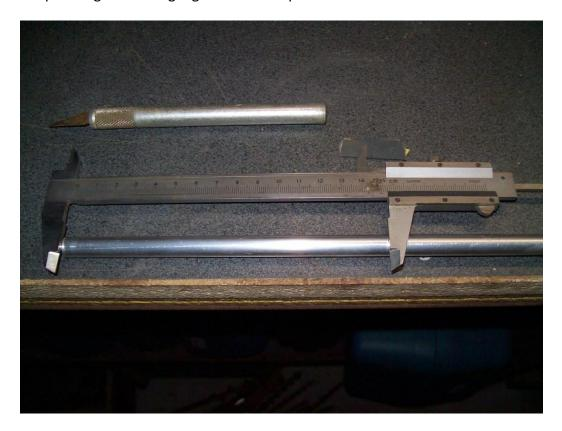
Cut a 'poofteenth' over length with a pipe cutter and dressed to length with a No2 flat bastard until it gauged up the right length with the vernier as set.
