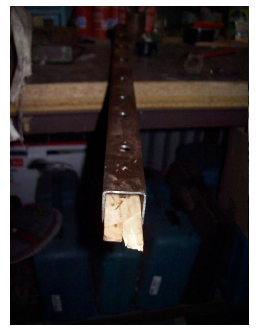
Shot of the jig with timber shims in place and the ferule set for the FME connector if you don't have or want to buy a crimping tool made using a 3/16 chainsaw file. Nice tight crimp.
